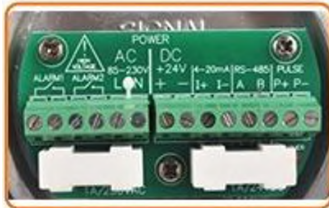
Double power supply system
